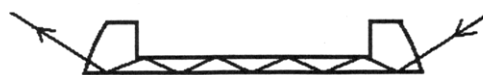
Figure 1. Schematic of the side view of a truncated ATR crystal with multiple reflection path illustrated.
